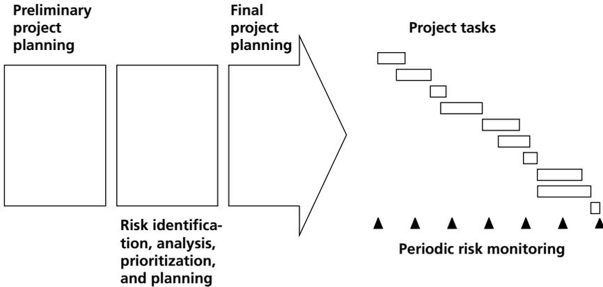
**Figure 13-2** Activities specific to risk management are shown at the bottom, and other project activities are listed at the top. During the project front end, the initial steps of risk management occur after initial planning but precede final planning, and during subsequent task execution, the risk-monitoring step occurs periodically
